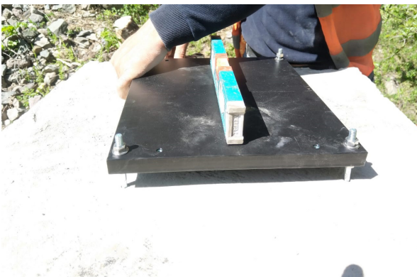
Figure 5. Leveling and sensor orientation (typically one axis of each accelerometer facing the same direction) are important aspect during installation process.
