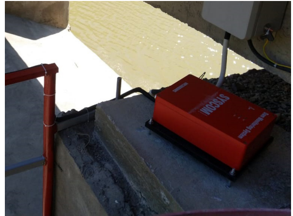
Figure 4. MR3000DMS MP1, master device on-structure, protected by the dam road bridge with a suitable device axis orientation.
