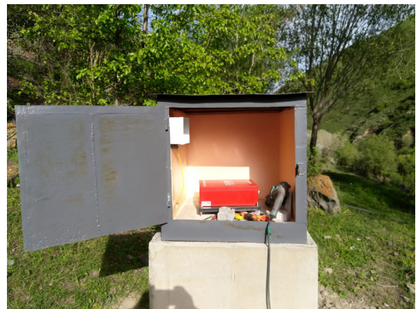
Figure 6. Protective housing for MP3 with concrete pad for proper coupling to the ground. The housing is grounded and therefore well protected against lightning.
