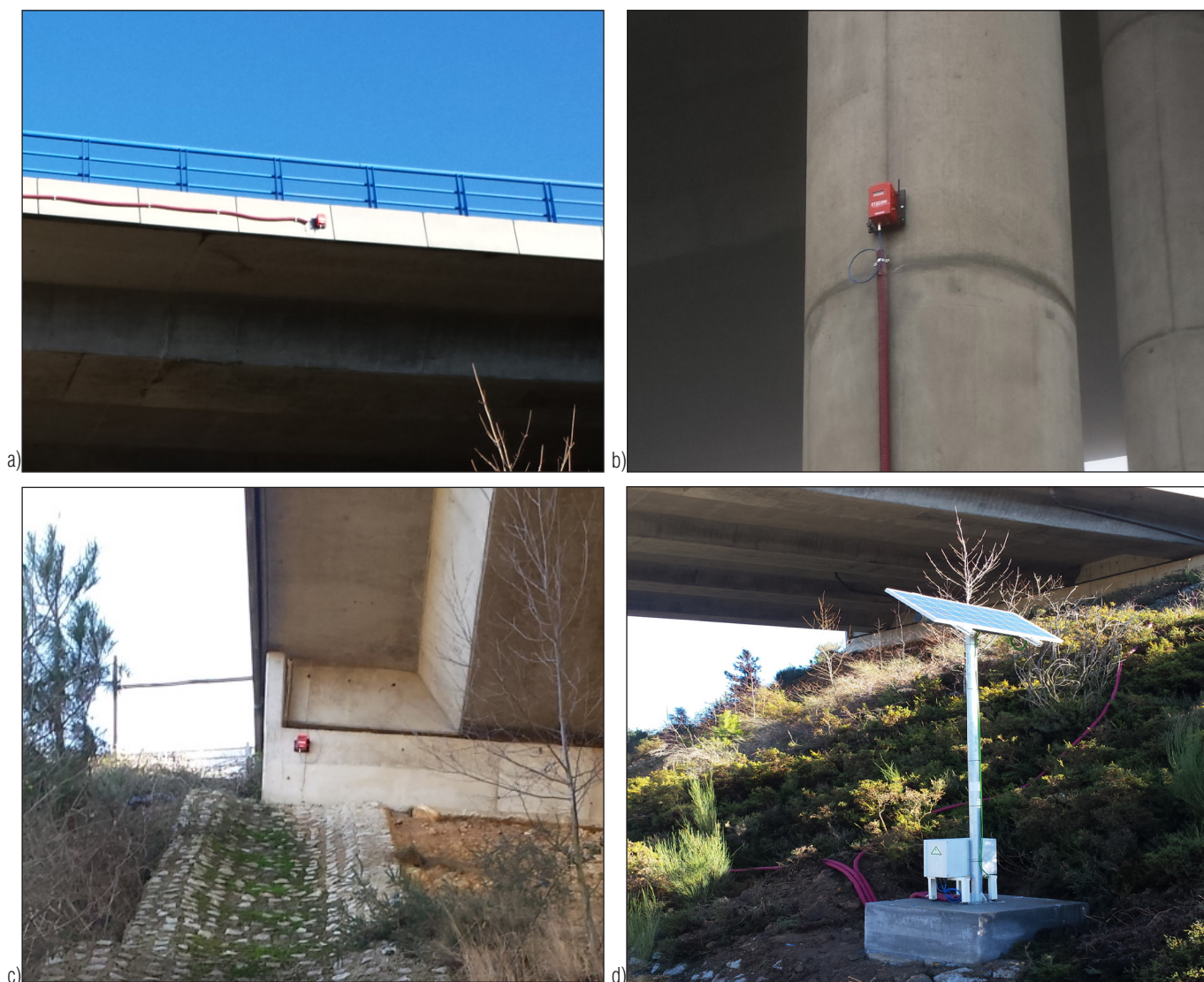
Figure 3. Instruments installed for the vibration monitoring of the A7 viaduto: a) MR1 on the external side of the bridge deck; b) MR2 on a pillar; c) M3 on the bridge abutment; d) solar panel and battery for the power supply of the MR3000C devices.
