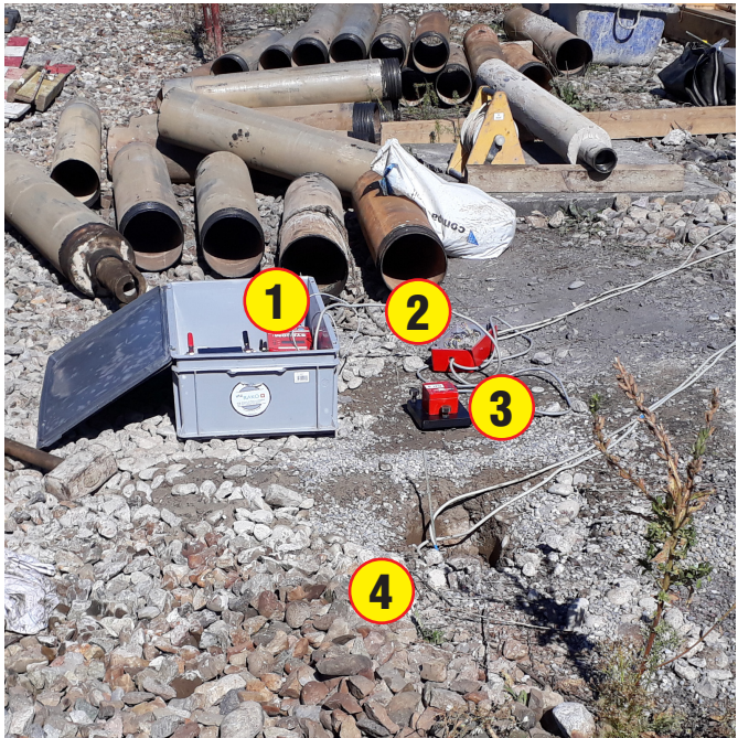
Figure 4. Measurement point MP1. 1) The recorder MR3000TR. 2) A junction box for the connection to the three external sensors. 3) The sensor at the surface. 4) The underground sensors.
