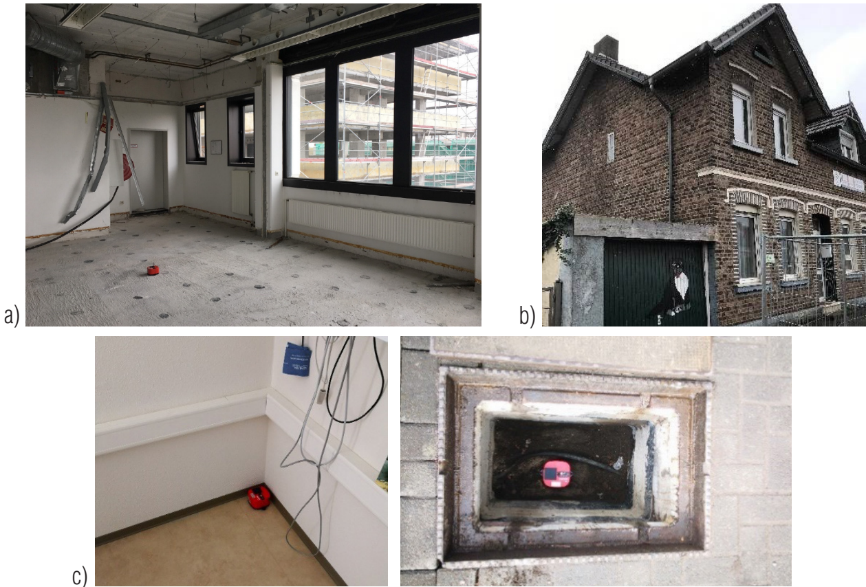
Figure 2. Real installations of the ROCK: a) in the vacant building close to the demolition monitoring; b) at the top of a house close to piling works; c) in the sleep clinic and inside the cable pit, for the monitoring of the construction site.
