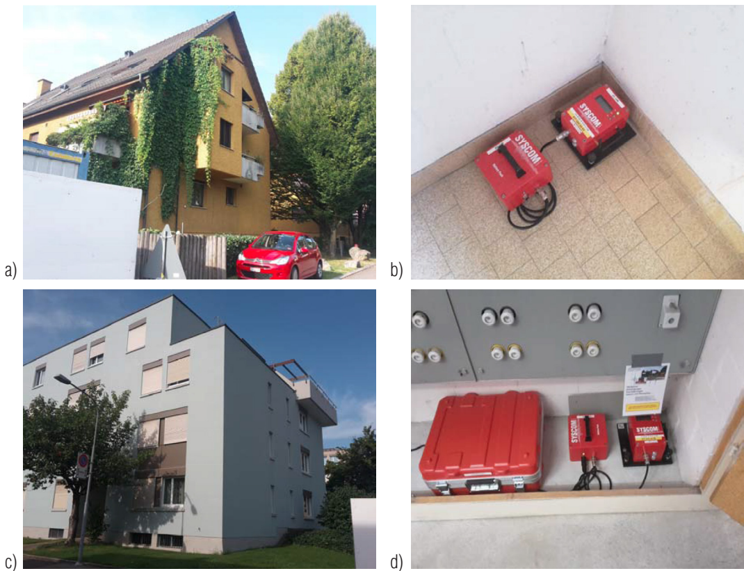
Figure 3. Building with measurement point MP1 (a) and the related MR3000C installed in the washroom, at foundation level (b); building with measurement point MP2 (c) and the related MR3000C installed in the electric cabinet, at foundation level (d).
