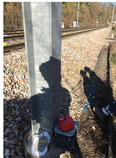
Figure 2. ROCK installed on a catenary pole
