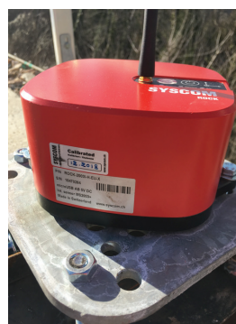
Figure 4. Stand-alone ROCK beacon, typical installation without cables
