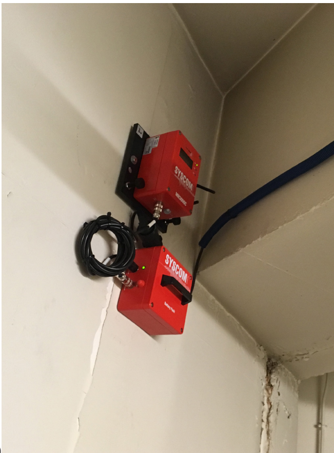
Figure 3. MR3000C installed in different locations in the T2A sector of the Grand Paris: on a warehouse wall, in vertical position (a); on a load-bearing wall inside a building, in vertical position (b) and at the foundation of a building, in horizontal position (c).
