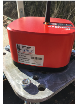
Figure 4. Stand-alone ROCK beacon, typical installation without cables
