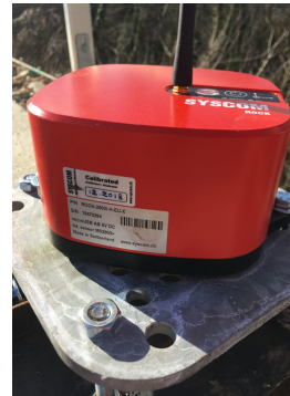
Figure 4. Balise ROCK autonome, installation typique sans câbles
