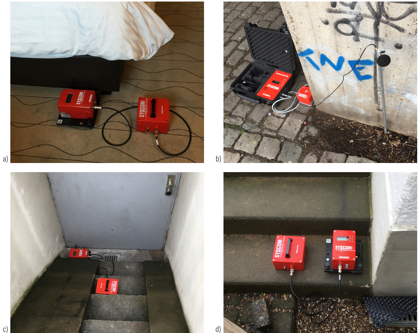
Figure 3. Instruments installed for the vibration monitoring: MR3000C in MP1 (a); MR3000BLA in MP2 (b), MR3000C in MP3 (c) and MR3000C in MP4 (d).
