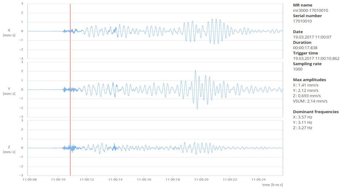
Figure 5. Time histories recorded in MPI, in the Bonn Marriott Conference Hotel, during the demolition of the Bonn Center.
