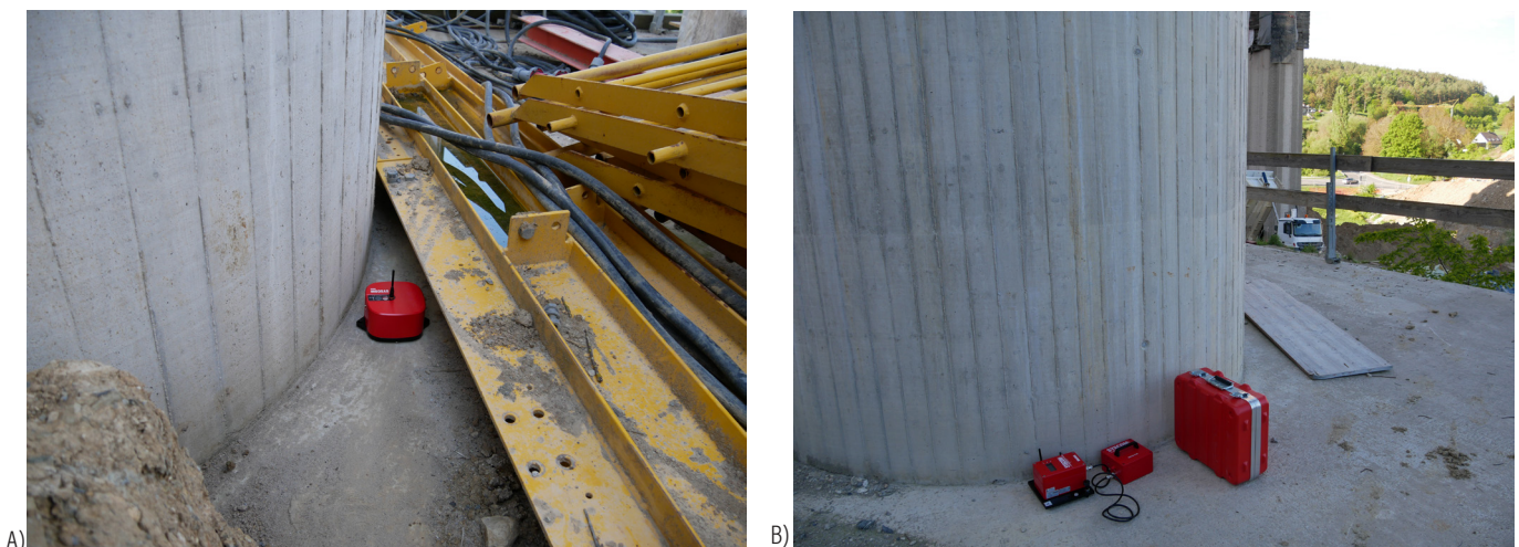
Figure 4. Instruments installed closed to piers of the new bridge: A) a ROCK. B) a MR3000C with its battery pack.
