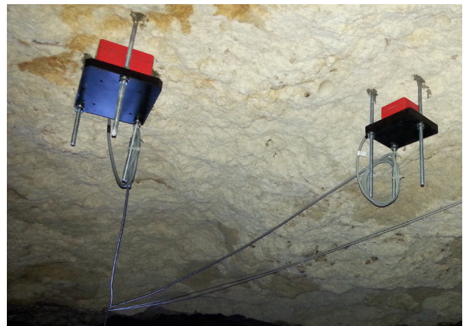
Figure 4. External velocity sensors MS2003+ installed at the ceiling of a cave, with MR3000C recorder installed in the above street, according to CONFIG. 5.
