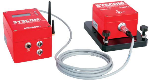
Figure 6. Syscom MR3000C with external MS2003+ sensor connected by a 3 m cable
