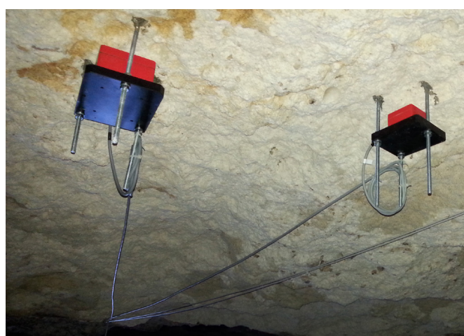
Figure 4. External velocity sensors MS20003+ installed at the ceiling of a cave, with MR3000C recorder installed in the above street, according to CONFIG. 5.
