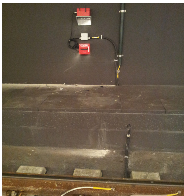
Figure 3. MR3000C with external battery pack installed on the tunnel wall inside an underground train station.
